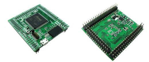
DUE-CORE is a compact version of DUE, It integrates all peripherals required for MCU, and all GPIO are connected to the 2.54mm connectors for users. As a standard MCU core board, apart from main features with DUE also has the following features:
