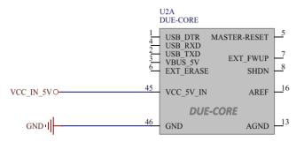
**Power Connection 3:** Both Programming port and VCC\_5V\_IN are connected , In this case , the VCC\_IN\_5V is priority, The connection as below :
