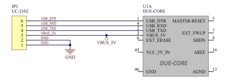
**Power Connection 2:** powered by VCC\_IN\_5V, in this case , The VCC\_5V\_IN must limit tolerance within +/-5% , which means the voltage range is 4.75-5.25V. The connection as below :
